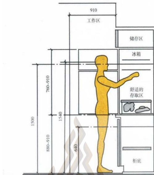
Figure 3.2 Data reference for cabinet
