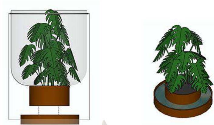
Figure 3.9 Rope to absorb the water, Water tank
