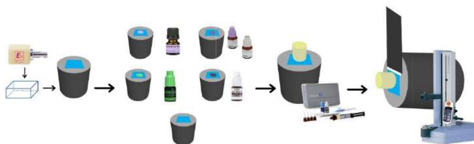
Figure 6. To assess the potential of chemical bonding, shear bond strength tests were performed on polished surfaces (N=50)
