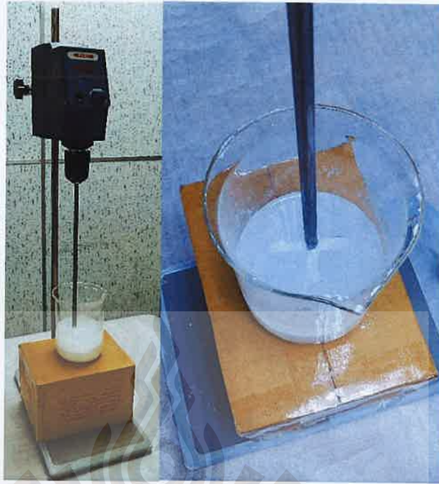
Figure 7 Mixing barium sulfate with resin by over-head stirrer.
