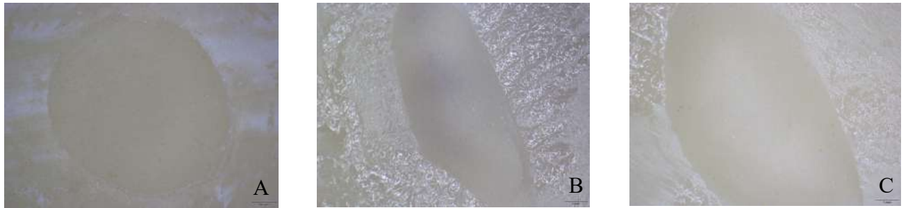
(Fig.8) The mode of failure. The stereomicroscope photographs above legends show representative failure modes for each corresponding type of failure on ceramic side. A: Adhesive failure, B: Mixed failure and C: Cohesive failure
