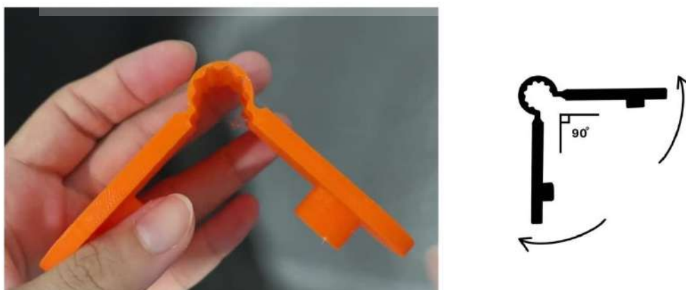
Figure 3.27 Experimental 3D printing techniques of connectors 02.
