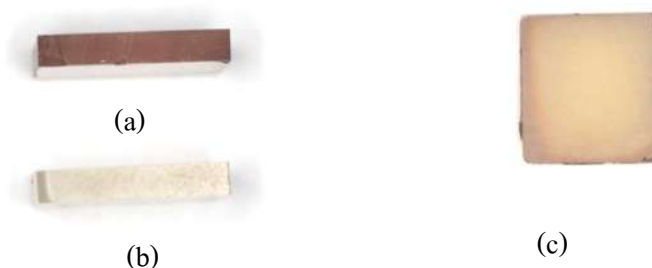
Fig.15 Specimen's corners after it was immersed in red wine of the controlled group where no surface treatment was done (a) compared with the area that was not immersed in red wine (b) and the area that has gone through surface treatment before it was immersed in red wine (c)
