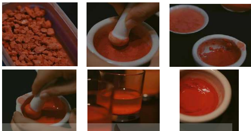
Figure 4.6 Water washing process
