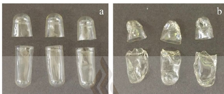
Figure 4.1 Physical appearance of (a) insoluble (exposed to formaldehyde vapor for 6 h) and (b) partially soluble crosslinked HGCs (exposed to formaldehyde vapor for 4 h) after being immersed in water for 24 h.
