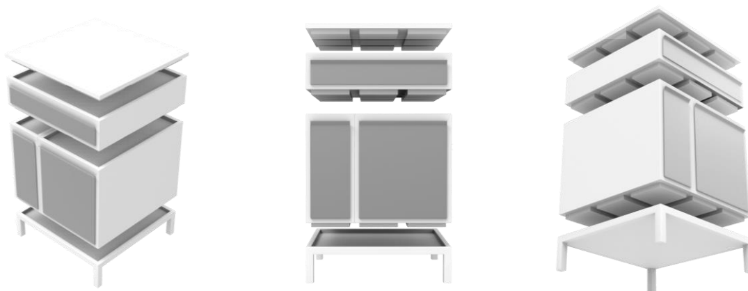
Figure 4.5 Exploded view of an add-on module joining system
