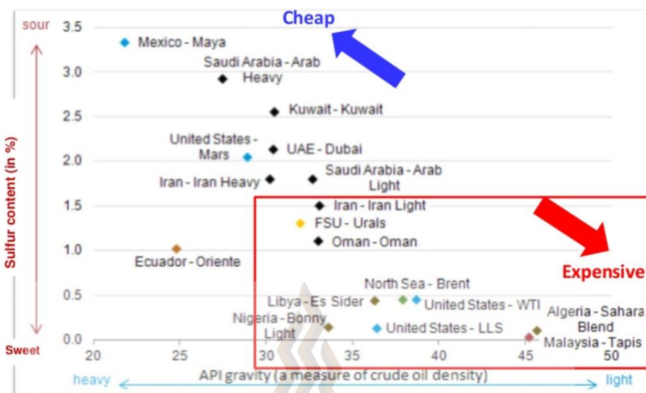
Figure 2: Density and Sulfur contents of selected crude oils
